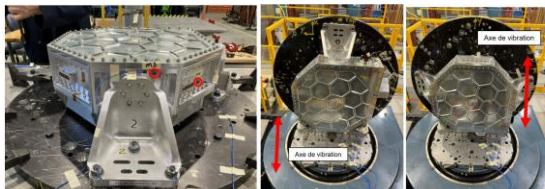
Figure 1. Shock/vibration test fixtures with the laser installed
